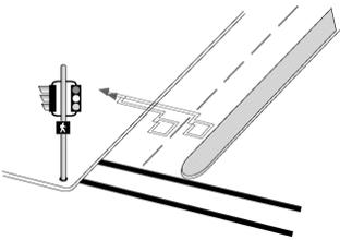
Detectors are devices for indicating the passage or presence of vehicles. In the past, these consisted of wire loops placed in the pavement at intersections. Today, video cameras are used to detect vehicles at traffic signals to change the operation of the signal to serve the heaviest vehicular traffic movements.
