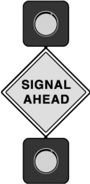
Flashing beacons (sometimes called flashers or flashing lights) are frequently requested in the belief they will slow down traffic. However, the real purpose of flashers is to attract attention to unexpected hazards in the roadway.
